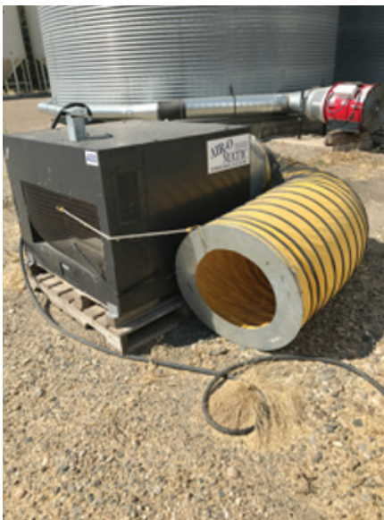
Fig. 10. Supplemental heat source to facilitate rapid drying of hemp grain. Photo Credit: Jeff Kostuik.
