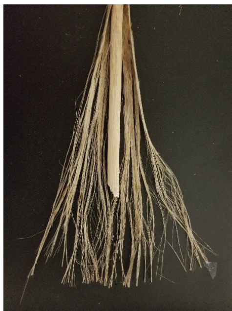
Fig. 4. Image of hemp stalk showing the bast fiber outer and woody core inner components (Permission: Sunstrand).
